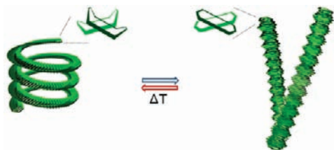
Figure 6. Schematic representation of reversible transformation of helical coils and straight rods of elliptical macrocycles.
